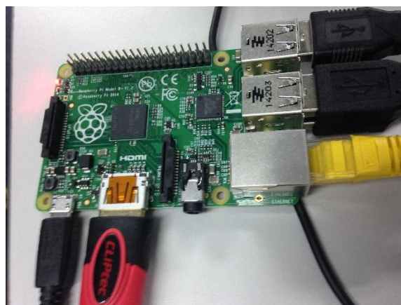
Figure 6: Raspberry Pi model B+ connected to HDMI, Mouse, Keyboard, LAN and XBee (USB)
