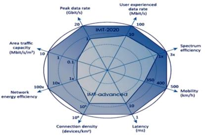
Figure 3 Enhancement of Key Capabilities from IMT-Advanced to IMT-2020[7]
