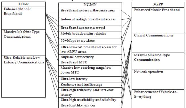
Figure 12 Comparisons of 5G Networks Services in ITU-R,3GPP&NG Mobile Networks
